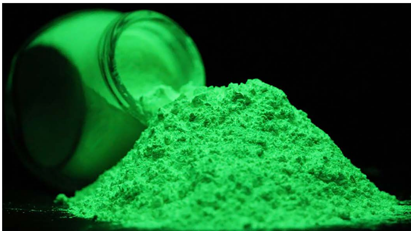
Figure 1. Copper-activated ZnS afterglow at 530 nm. Application limiting drawbacks include sensitivity to moisture over time and short afterglow time and rapid decrease in intensity after only a few hours. Enhancement of afterglow intensity by incorporation of a large amount of dopant (activator) negatively affects both mechanical and physical properties leading to a rapid degradation in chemical stability.
