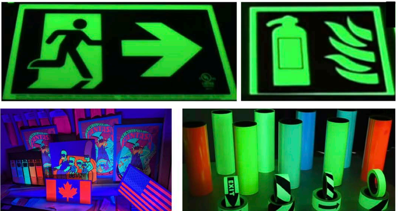
Figure 4. Typical examples of persistent-phosphor incorporation in self-luminous way-finding and emergency signage, novelty self-luminous printing and self-luminous polymer film.
